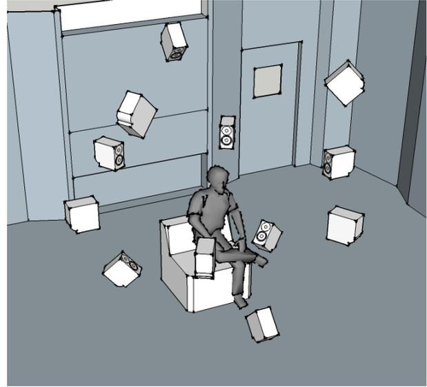
Figure 2: 3D model of the speaker layout used for the height listening test
