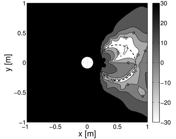
Figure 2: Magnitude in decibels of the sound attenuation with a spherical secondary source designed to minimize the total pressure on a sphere centered at  $(r, \theta, \phi) = (0.5m, 90^\circ, 0)$ ; the primary sound field is as in Fig. 1.
