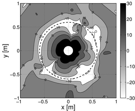
Figure 6: Magnitude in decibels of the sound attenuation with a spherical secondary source designed to minimize the total pressure on a shell shape at  $r = 0.6m$  around the source, and the primary sound field as in Fig. 1.
