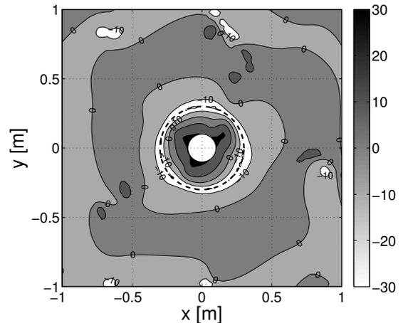
Figure 8: Magnitude in decibels of the sound attenuation with a spherical secondary source designed to minimize the total pressure on a shell shape at  $r = 0.3m$  around the source, the primary sound field as in Fig. 1.
