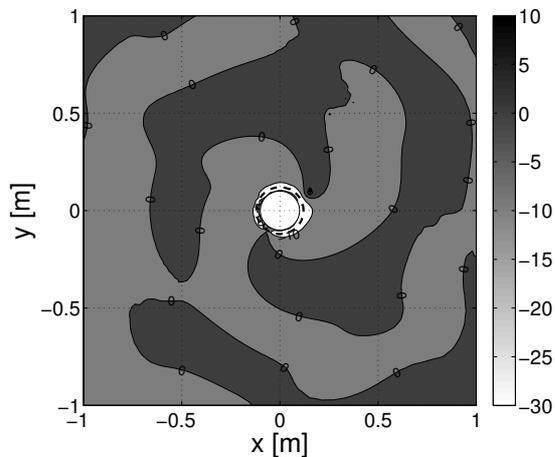
Figure 9: Magnitude in decibels of the sound attenuation with a spherical secondary source designed to minimize the total pressure on a shell shape at  $r = 0.12m$  around the source, and the primary sound field as in Fig. 1.
