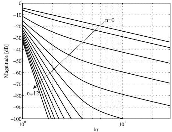
Figure 7: Magnitude of  $h_n(kr)/h'_n(kr_0)$  for  $n = 0, 1, \dots, 12$  as a function of  $kr$ , for  $kr_0 = 0.916$ .
