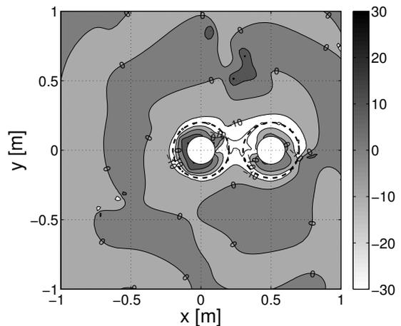
Figure 10: Magnitude in decibels of the sound attenuation with two spherical secondary sources, designed to minimize the total pressure on the shell around each source; the primary sound field as in Fig. 1.
