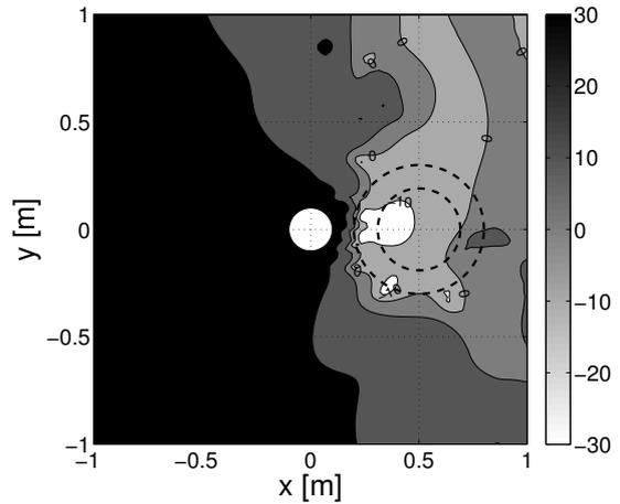
Figure 5: Magnitude in decibels of the sound attenuation with a spherical secondary source designed to minimize the total pressure on a dual sphere centered as in Fig. 3, the primary sound field as in Fig. 1, but source order is reduced to  $N = 4$ .
