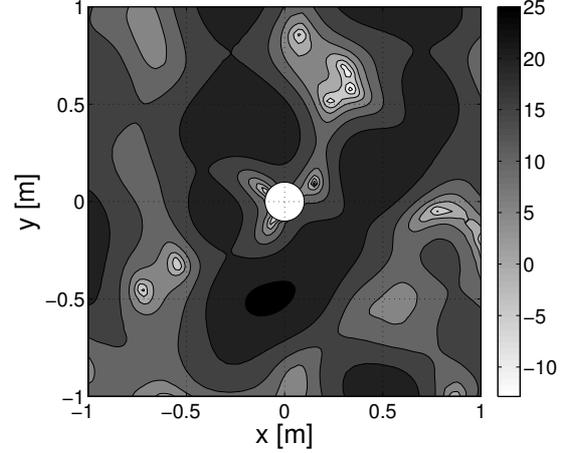
Figure 1: Magnitude in decibels of a multiple plane-waves primary sound field with secondary source switched off.
