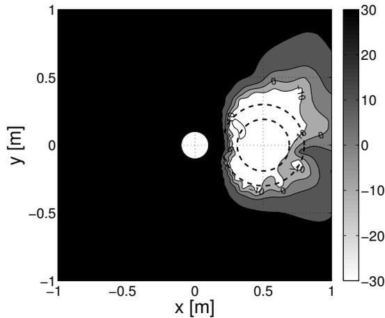
Figure 3: Magnitude in decibels of the sound attenuation with a spherical secondary source designed to minimize the total pressure on a dual sphere centered as in Fig. 2, the primary sound field as in Fig. 1; source order is  $N = 12$ .
